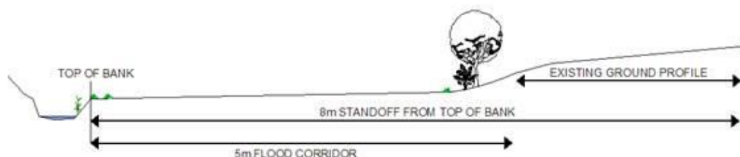
Figure 3.1 - Typical cross section of enhanced flood corridor.
