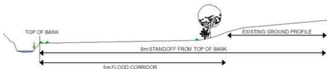
Figure 5.1 - Proposed flood corridor expansion, indicative cross section
